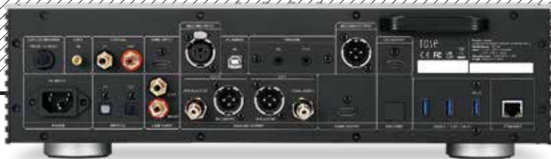
ABOVE: Wired/optical and wireless (via USB dongle) Ethernet inputs, are joined by coaxial and AES/EBU (to 384kHz/DSD128 DoP), optical (to 192kHz/DSD64 DoP), iS/HDMI and USB-B (to 768kHz/DSD512) plus two USB-A ports for external media (an internal bay accommodates users' own SSD/HDD hardware). RCA line ins are joined by RCA/XLR line outs, HDMI (video and iS) outs, coax/opt outs and 12V trigger ports
